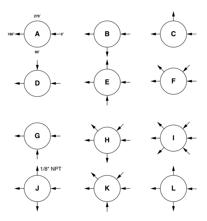
LOCATION OF PORTS FROM TOP VIEW ARROW POINTING TOWARD BODY IS INLET ARROW POINTING AWAY FROM BODY IS OUTLET
